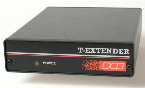
Since a T-1 line is bi-directional, T-Extenders are most always used in pairs. When the length of line is greater than about 5,000 feet, additional T-Extenders must be inserted along the line each 4,000 to 5,000 feet.
