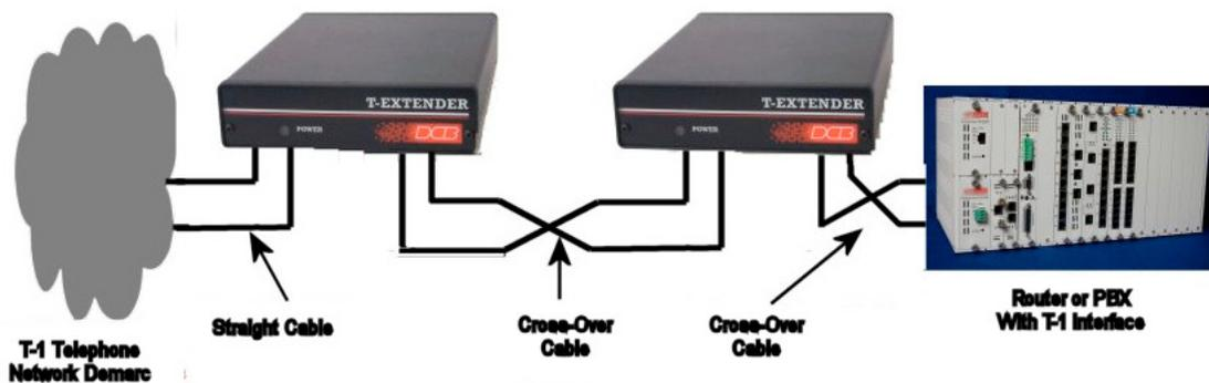
1. Plug a straight cable between the first T-Extender and the smart jack using the "to TELCO" adapter.
