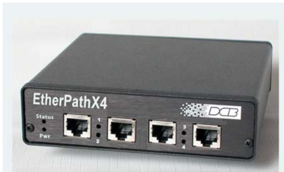
Front of EtherPathX4 showing the 4 serial ports
